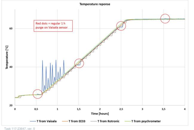
Note stepwise behaviour of **Rotronic sensor**
