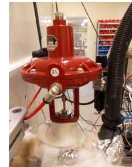
Heated valve at exit of pressure chamber
