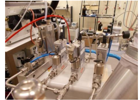
Flow mixing using mass flow controllers
