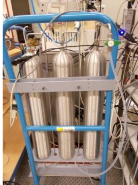
Saturators automatic refill from external containers at 23 °C. (11 l water, allowing 24 hours operation at 150 °C and 95% rh)
