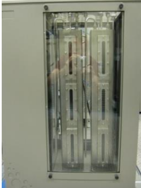
Mineral oil bath for dew-point temperatures up to 150 °C
